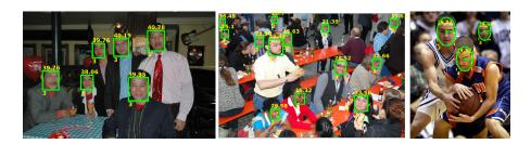
Figure 6: Qualitative detection results for the AFLW/PASCAL experiment (first image), AFLW/AFW experiment (second image), AFLW/FDDB experiment (last image). We display faces with score≥10. Over each detection and under the face we show in yellow, respectively, the score and the estimated face class. In the FDDB results, we show in green the estimated ellipse from the yellow rectangle detection.
