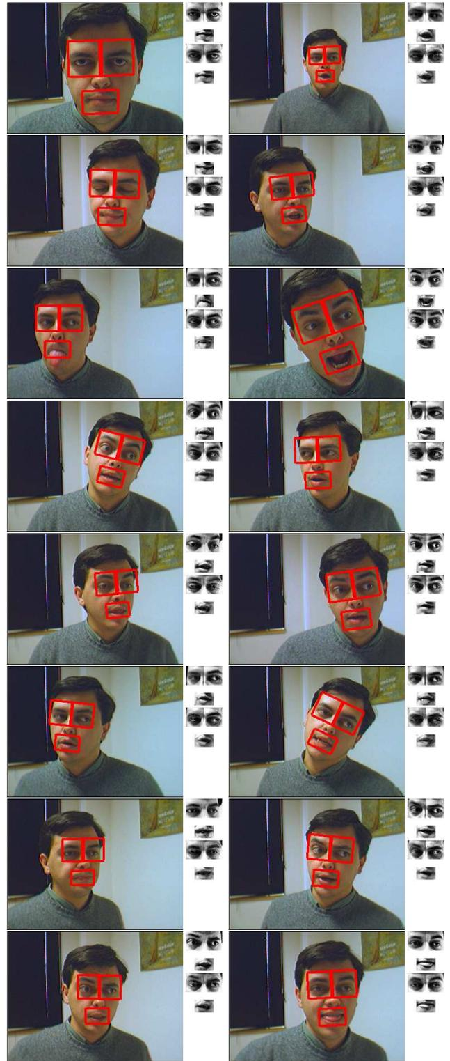
**Figure 4. Rotation-translation-scale modular appearance based tracking. Results for a 4787 image sequence. Half of the sequence was used in training (2720 images) and the other half for tracking (2067 images).**
